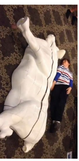
Lifesize 3D Printed (half) Cow designed by Portland 3D Printing Lab member Mazuir Ross. Cow consists of 99 separate pieces and required over 700 hours to print on 14 different 3D printers. 11 year old Paul poses with the cow to show its size. ( https://3dprint.com/63136/3d-printed-cow-portland )
